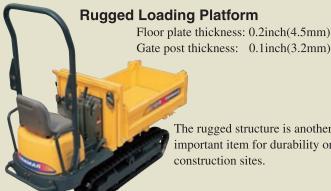
The rugged structure is another important item for durability on construction sites.
